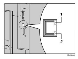
1. Yellow: lights up when 100BASE-TX is being used. Turns off when 10BASE-T is being used.
