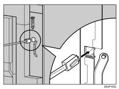
Connect the other end of the cable to the network, such as a hub connection.
