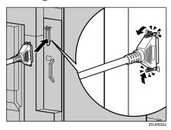
3 Attach the other end of the parallel cable to the port of the computer. Secure the cable.
